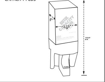
placement, dispensers should be mounted at least 3" above any countertop, fixture or obstruction and at least 2" below any upper cabinet, fixture or obstruction.
